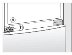
■ Fit hinge pin ⑨ into middle hinge plate ① in the lower door.
